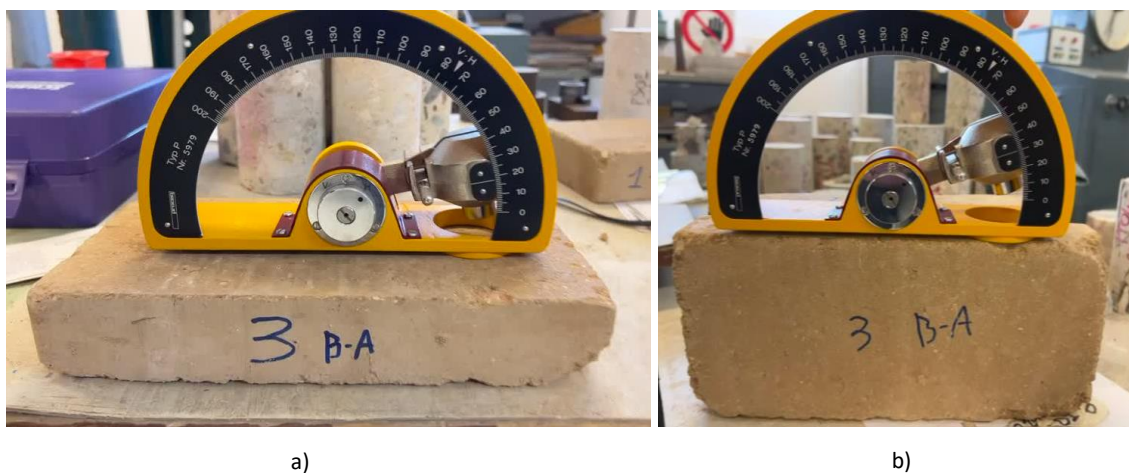
Figure 8. Sclerometric tests: a) B-face, and b) F- face.
