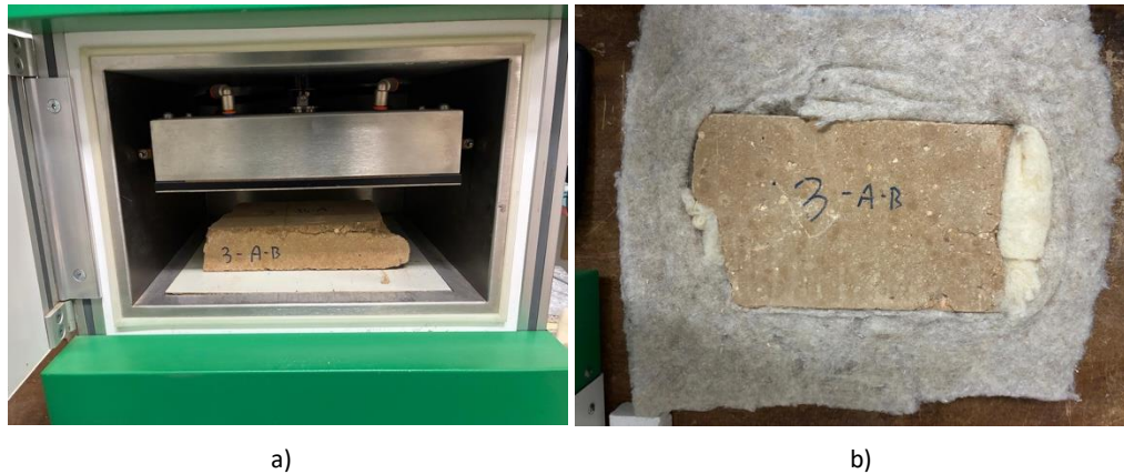
Figure 4. a) Measuring chamber of the heat flow meter, and b) sample with the heat guard.
