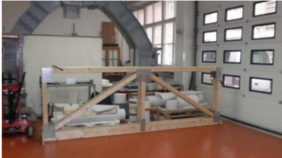
Figure 1. Timber truss prepared for experimental testing, photograph from the original experimental programme (Čizmar 2012).
