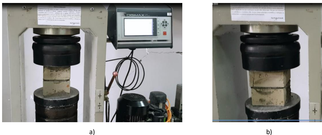
Figure 13. a) Sample during testing, b) Sample after testing.
