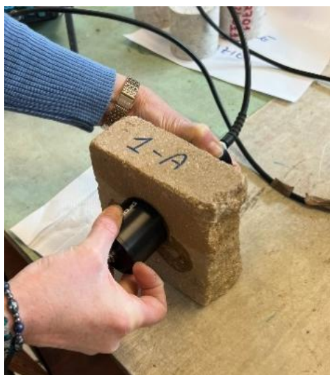
Figure 7. Samples during the ultrasonic test, along the path, Height (H).
