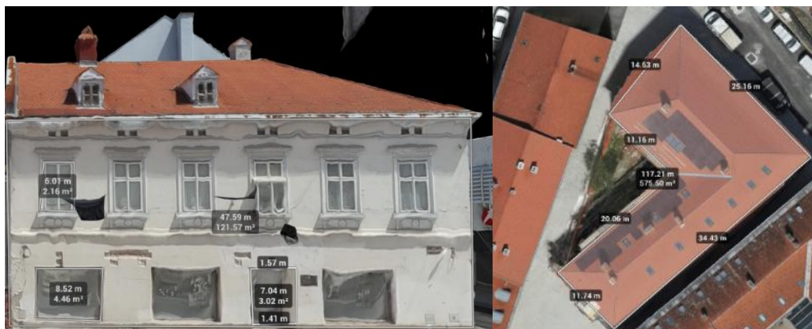
Figure 10. UAV-based LiDAR and photogrammetric data acquisition for a geometry.
