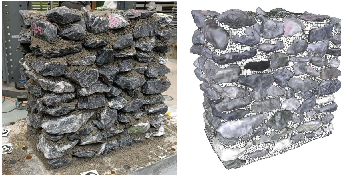
Figure 11. (left) Physical stone masonry wall; and (right) geometrical DT [253].
