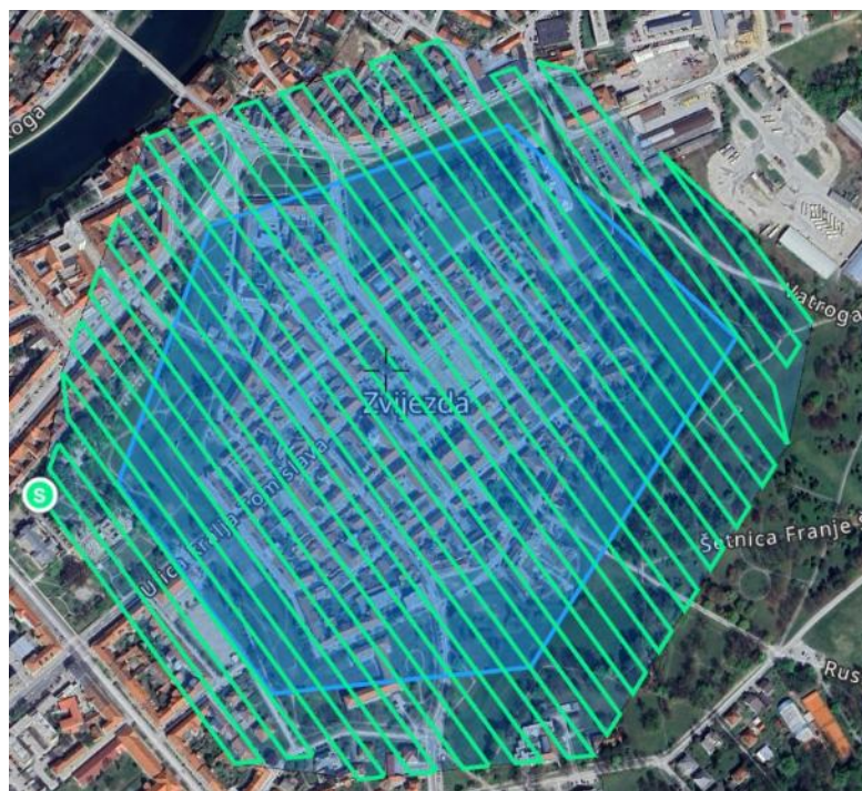
Figure 5. An example of a predefined UAV flight path for a photogrammetric survey mission.
