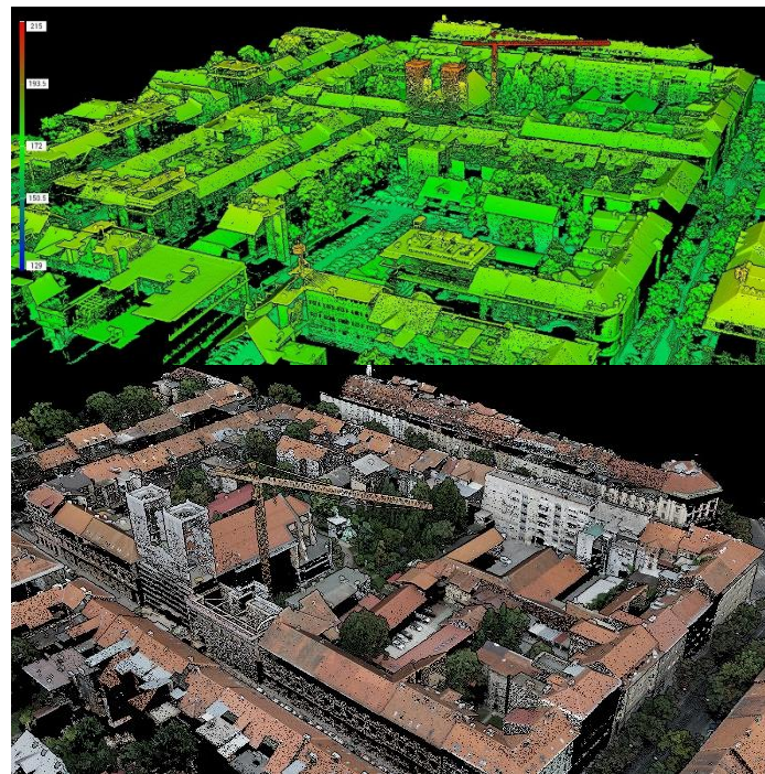
Figure 9. (top) Point cloud of 3 building blocks obtained by a LiDAR system (green colour – lower altitude, red colour - higher altitude); (bottom) more detailed view of the point cloud of one building block.
